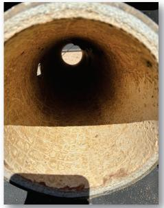
Sample taken from recent repair of cement mortar lined/coated (CMLC) steel pipe in Avocado Street.
