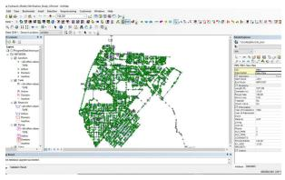
Mesa Water's hydraulic model is in Innovyze's InfoWater and is used for hydraulic evaluation of Mesa Water's distribution system.
