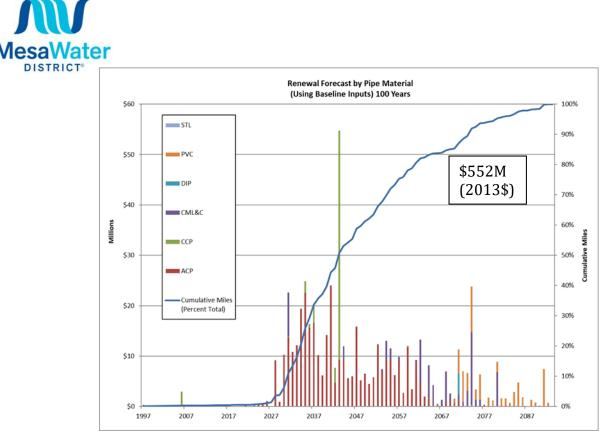
Figure 1. 100-Year Age-Based Pipeline Replacement Curve, 2013.
