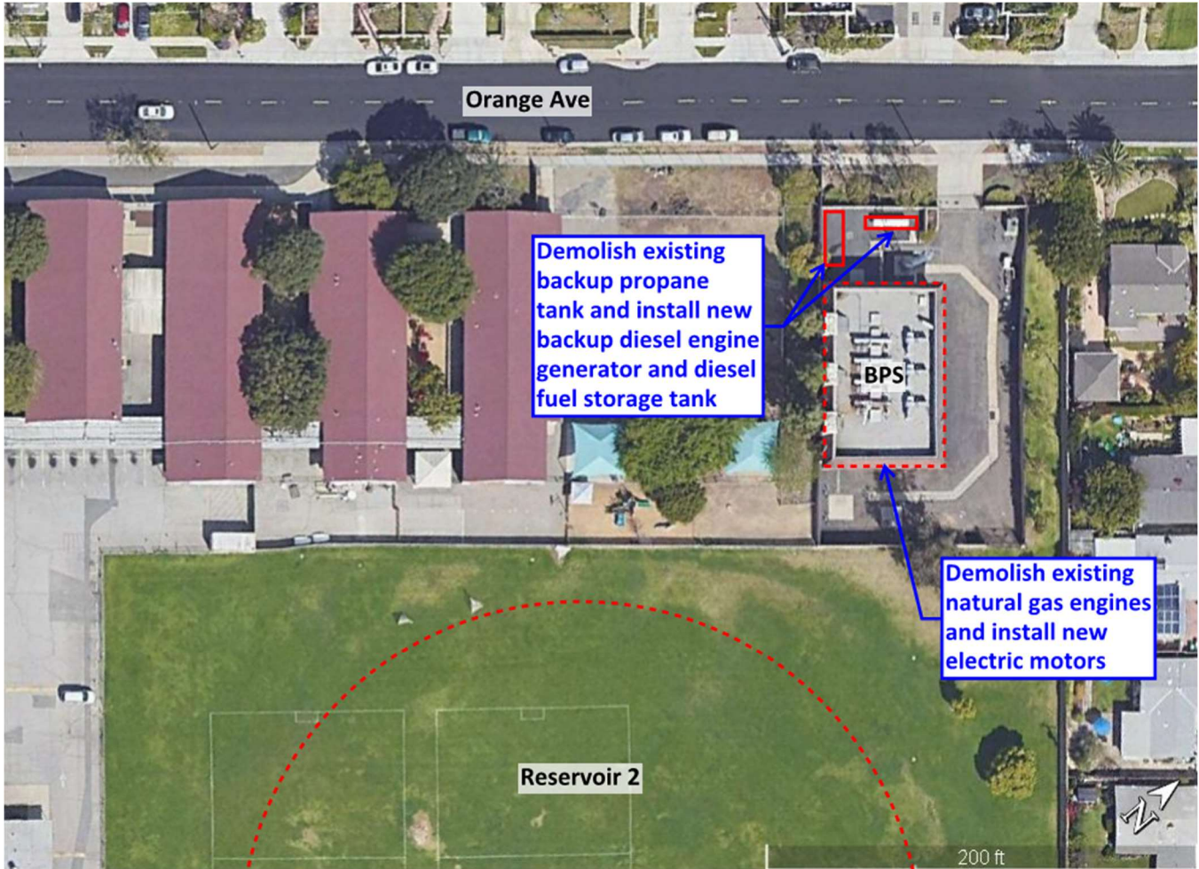
Figure 11-2. Reservoir 2 Proposed Diesel Fuel Supply
